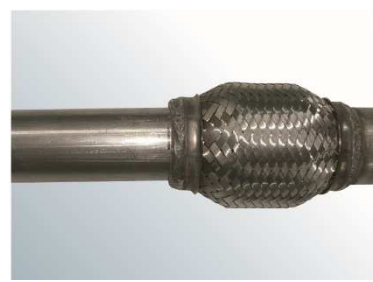
4. – 6. Insert connecting pipe into the new flexible tube to a depth of about 10 mm and then weld it.
