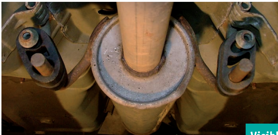
Natural rubber (left) and EPDM (right) in direct comparison: long-term test on the centre silencer of an Opel Corsa C.
